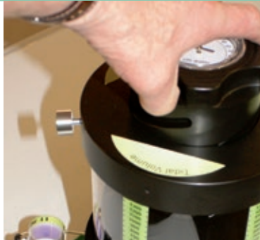
Tidal volume control with twist screw
